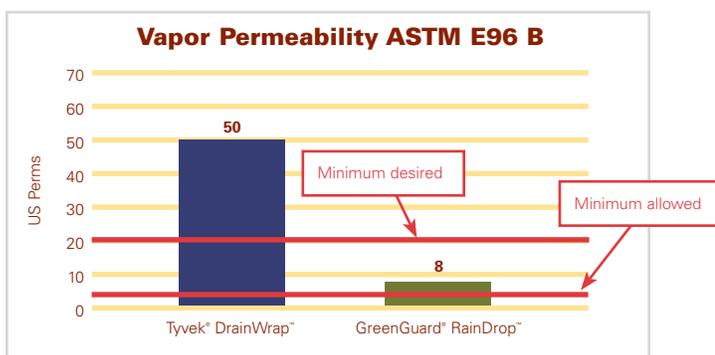
\*The minimum value established by code for this test method is 5 perms. The minimum desired value is based on studies showing that at levels below 20 perms the natural drying rate of components starts to be impacted negatively.
