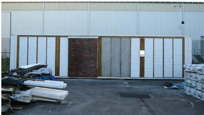
Relocatable Building Enclosure Test Station (RBETS) units were designed and built to test wall assemblies and their component materials in a variety of climates.
