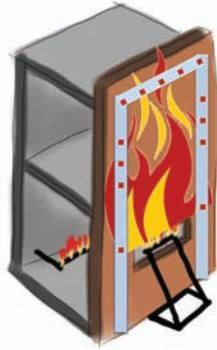
Inside wall assembly, thermocouples shall not exceed 1,000°F during the 35-minute test.
