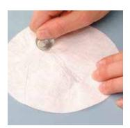
Tyvek° is not abraded. Barrier is not compromised.
