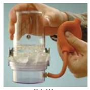
**Air bubbles** Air flows easily with Tyvek\*.
