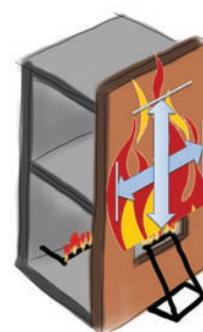
Externally, flames shall not reach 10 feet above the window's top.
