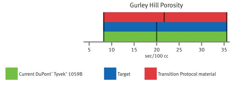
Transition Protocol typical values represent data from 100 rolls across different line and polymer combinations from a limited number of manufacturing campaigns. Values will be refreshed, as necessary, upon data collection from additional campaigns and long-term variability discernment.
