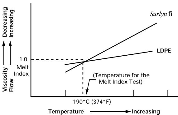
Often, molding cycle time dictates use of the minimum melt temperature. **A higher than minimum melt temperature is recommended if optimum physical properties are to be achieved in the molded part.** To produce parts with maximum impact performance and freedom from weak weld line zones, always use a mid-range or high melt temperature with some sacrifice of cycle time.
