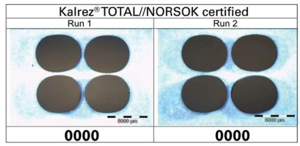
Tested according to Norsok M710 rev2 standard (K312 (15.24x5.33mm) O-ring; 67% groove fill; Test gas 10% CO2 in methane)
