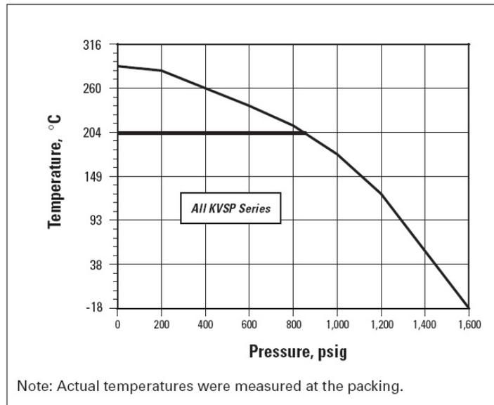
**Figure 7. High-Temperature Applications—The Effect of Standard and Extended Stainless Steel Bonnets on the Temperature at the Packing in Control Valves**
