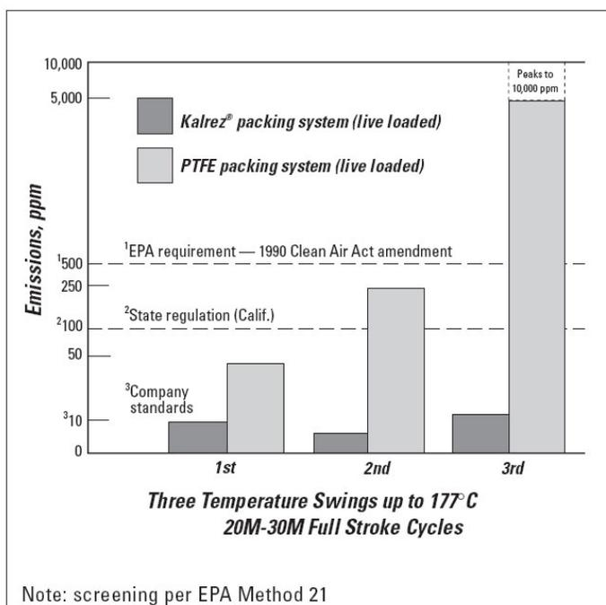
Until now, conventional packing materials and packing systems have not been able to provide the lower leakage rates provided by the metal bellows. The DuPont™ Kalrez® packing systems offer a viable option in both absolute fugitive emission reduction levels and long-term performance.
