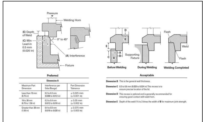
Figure 2. Ultrasonic Welding – Energy-Director Joint
