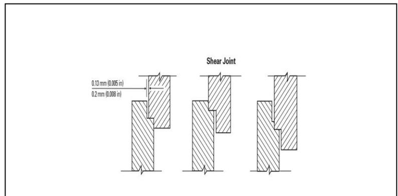
The major advantage of vibration welding is the ability to weld large, complex parts—to 0.61 x 0.46 m (2 x 1.5 ft.) in specially designed equipment. The weld area is not restricted to the periphery. Internal surfaces such as dividers or supports are easily welded with proper design and welding fixtures.
