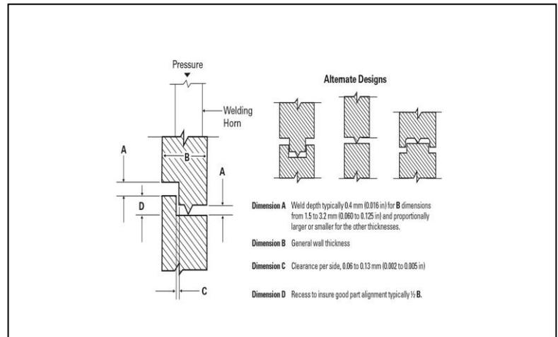
Figure 3. Flash Traps for Shear Joint
