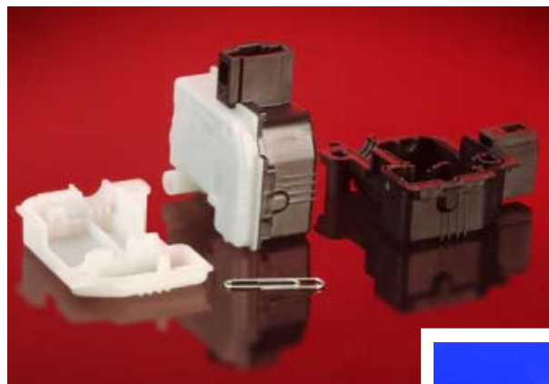
In automotive door lock (left) and fuel vapor canister (below), covers made of natural, laser-transparent PA66 are welded to black, laser-absorbing PA66 housings. Both materials are DuPont™ Zytel® nylon resins.
