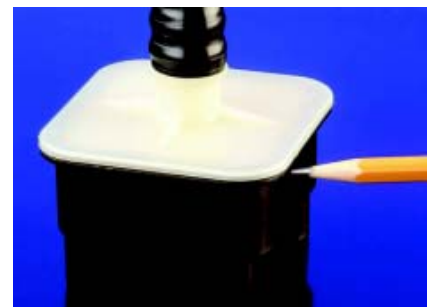
In automotive door lock (left) and fuel vapor canister (below), covers made of natural, laser-transparent PA66 are welded to black, laser-absorbing PA66 housings. Both materials are DuPont™ Zytel® nylon resins.
