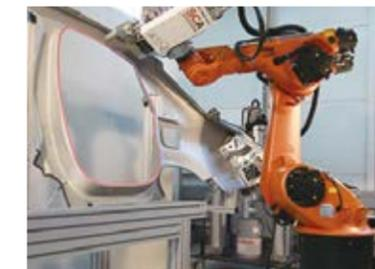
DuPont™ BETAMATE™ structural adhesives used to bond body structures
