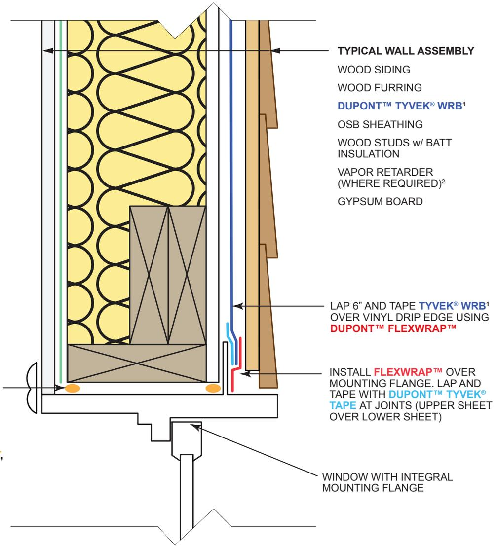
INSTALL TOWER® RESIDENTIAL SEALANT OR RECOMMENDED SEALANT (AND BACKER ROD AS NECESSARY) AROUND THE WINDOW OPENING AT THE INTERIOR. IT IS ALSO ACCEPTABLE TO USE **GREAT STUFF PRO™ WINDOW & DOOR POLYURETHANE FOAM SEALANT**, OR RECOMMENDED FOAM
