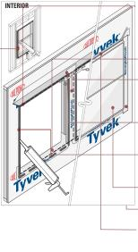
"I" cut WRB at rough openings with continuous horizontal cuts at head and sill. 45° cuts at window head extending min. 8" from corners. Flaps at jambs folded into the opening and secured. Head flap flipped up and secured. DuPont<sup>™</sup> FlexWrap<sup>™</sup> NF installed at each sill
