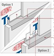
DuPont<sup>™</sup> Tyvek<sup>®</sup> WRB installed across wall so top edge of WRB is at bottom of beam. Two pieces of DuPont<sup>™</sup> Tvvek<sup>®</sup> WRB installed on either side of beam and sealed with DuPont<sup>™</sup> Tyvek<sup>®</sup> Tape. The two pieces extend min. 7" above top of beam and overlap lower WRB course min. 6"
