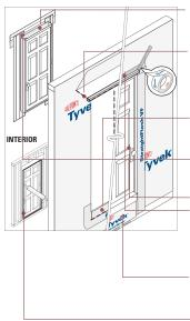
DuPont<sup>™</sup> StraightFlash<sup>™</sup> VF applied to interior side of door frame along jambs and head (head piece installed first).
