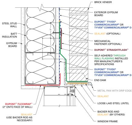
FLOATING LINTEL WITH METAL PAN AND MECHANICALLY ATTACHED THROUGH WALL FLASHING (SIDE VIEW)
