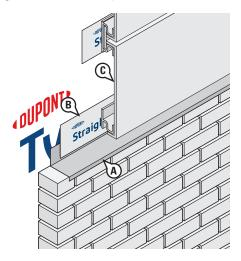
A. Install the "Z" or "L" metal flashing over the lower façade and onto the **Tyvek® WRB** with mechanical fasteners.
