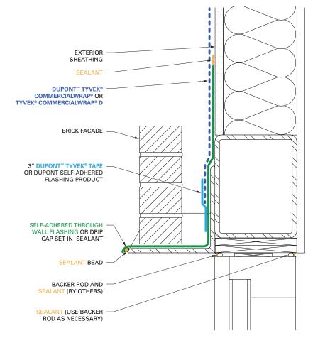
FLOATING LINTEL WITH THROUGH WALL FLASHING ADHERED TO DUPONT™ TYVEK® WRB (SIDE VIEW)
