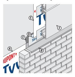
A. Install the first course of **Tyvek® WRB** so it extends a minimum of 2" **BEYOND** where the top edge of the lower façade will be located.
