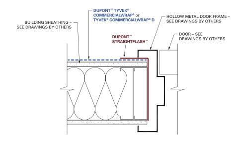
HEAD DETAIL (SIDE VIEW) - HOLLOW METAL DOOR
