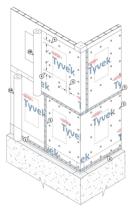
It is important to maintain the continuity of the **DuPont™ Tyvek® WRB** from top to bottom with proper shingling and overlap. The entire wall surface shall be wrapped, including unconditioned spaces.
