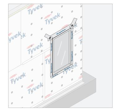
Windows aligned with the exterior finished wall typically require wood bump out framing around the window rough opening as shown in **Example 1**. The wood bump out framing is flashed and integrated with **Tyvek**<sup>®</sup> **CommercialWrap**<sup>®</sup> or **Tyvek**<sup>®</sup> **CommercialWrap**<sup>®</sup> **D**.
