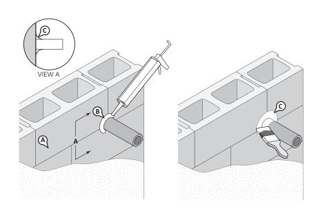
Option 2: Using DuPont<sup>™</sup> FlexWrap<sup>™</sup> EZ for Non-Flanged Products with Outer Diameter (OD) GREATER Than 2 Inches\*
