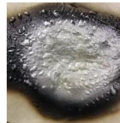
After 30 minutes direct flame (flame side)
